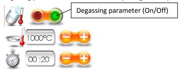
When turned ON this parameter will allow to execute the degassing function. If the degassing temperature is 10°C below the one of step 4 (or more), the door will open to reduce temperature more efficiently. Once the temperature is reached, the duration timer of degassing function is started. Then, the temperature of step 4 is reached again before the pouring is executed. During all degassing function, rocking speed and rocking angle parameters of step 4 are used.
